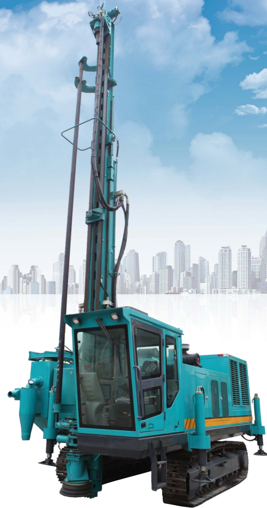
SWD DOWN-THE-HOLE DRILLING RIG
